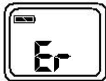
For all other error messages, it is necessary to reset the NU-263. To reset the NU-263, turn the unit off, remove the battery and wait for a minimum of one minute, reinsert the battery and turn on. If the error message remains, please contact the Service Dept. for further assistance.
