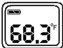
'Battery OK' : Measurements are possible
