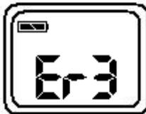
'Er2' is displayed when the NU-263 is exposed to rapid changes in the ambient temperature. 'Er3' is displayed when the ambient temperature of the unit exceeds 14°F (-10°C) or 122°F (50°C). In both cases, you should allow plenty of time (minimum 30 minutes) for the NU-263 to stabilize to the working/room temperature 32°F (0°C) to 104°F (40°C)
