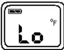
'Hi' or 'Lo' is displayed when the temperature being measured is outside of the range of the instrument. 'Hi' when higher than +428°F (220°C) and 'Lo' when lower than -27°F (-33°C)
